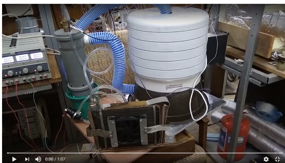
Fig. 2. Physical model of a condensation chamber for drying fruit and vegetable raw materials using a thermoelectric heat pump
