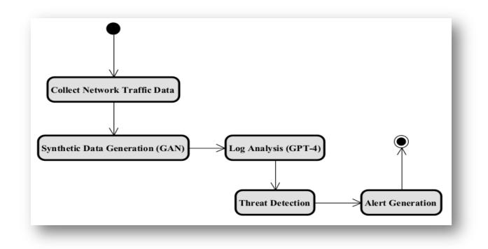
Fig. 1. Workflow of GenAI in Threat Detection
