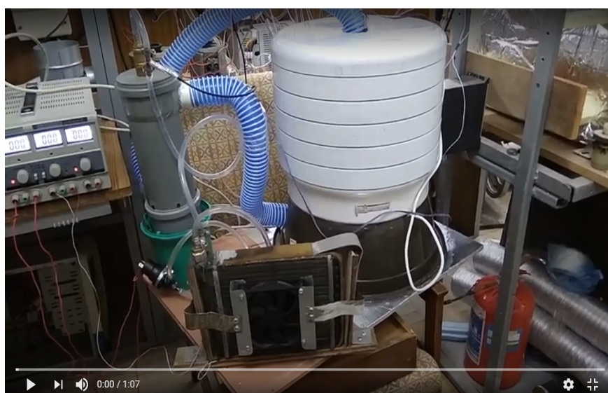
Fig. 2. Physical model of a condensation chamber for drying fruit and vegetable raw materials using a thermoelectric heat pump.
