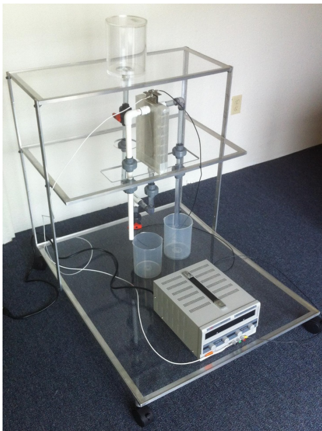
Fig. 5. Photograph of the System for Real-Time Adjustment of Acidity and Alkalinity in Deionized Water
