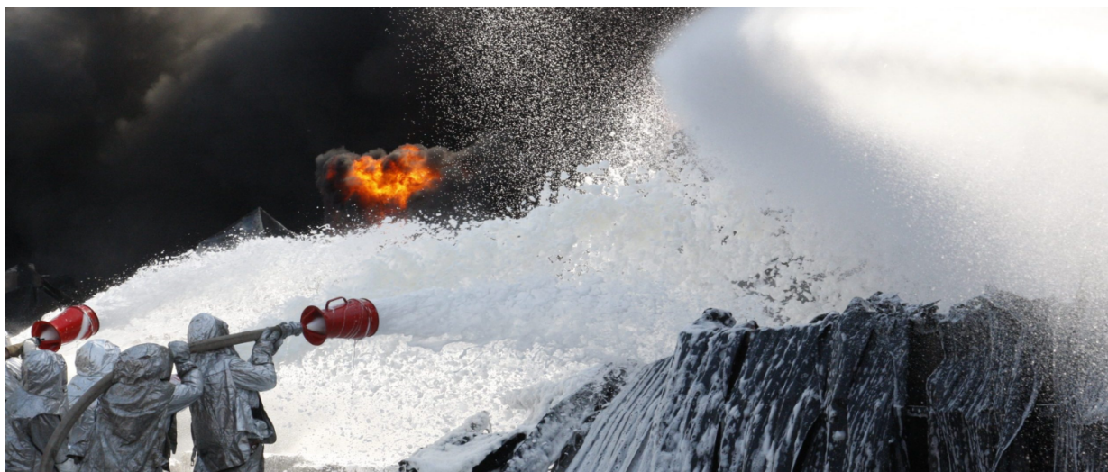
Fig. 1. Use of high-multiplicity foam generators for fire-fighting purposes
