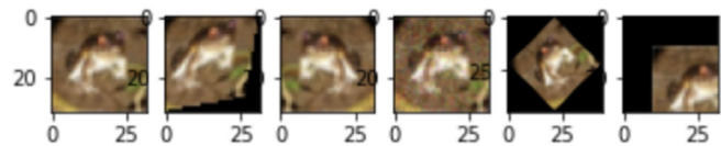
Fig. 1. Perturbation example. Left to right: original image, skew, mirror, white noise, rotate, translate
