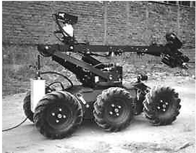
Fig. 5. Robotic remote-controlled complex on a wheelbase
