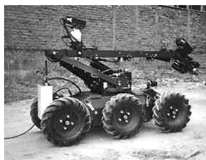
Fig. 5. Robotic remote-controlled complex on a wheelbase
