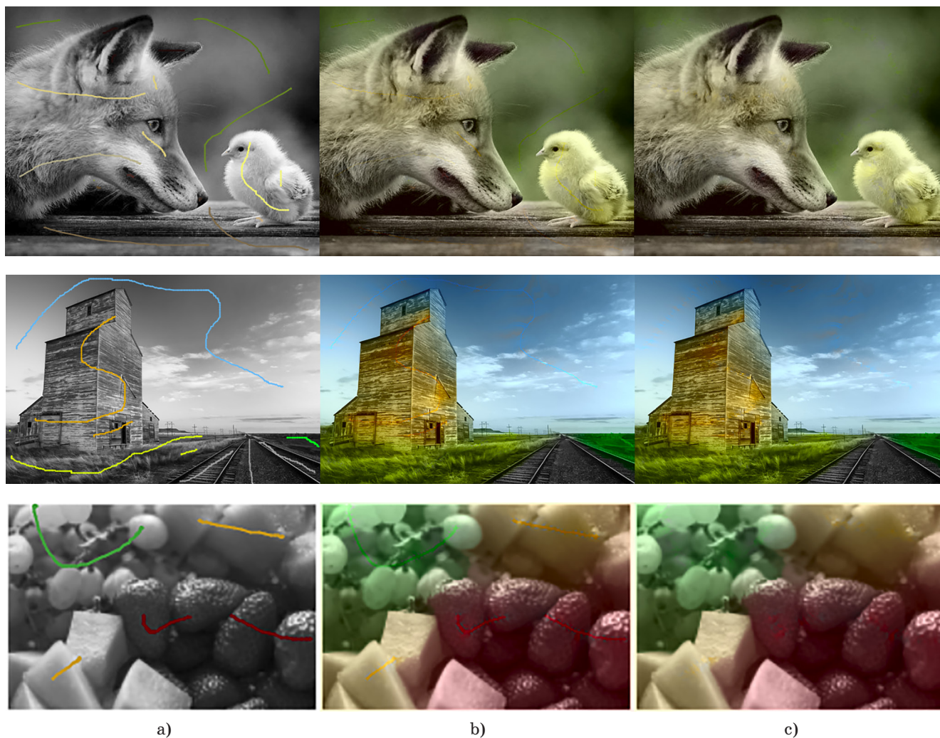
Fig. 11. Comparison of images during the repeated colorization algorithm execution. a) black and white images with markers; b) colored images after the first iteration; c) the same image after the second iteration
