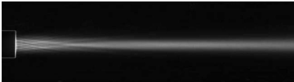
Fig. 2. A picture of an ultrasound wave emitted by a piezoelectric crystal at a frequency of 1.25MHz (after Guglielmi al., 2009) [3].
