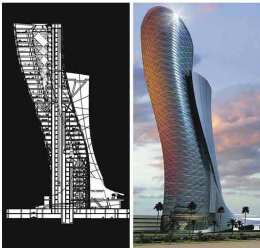
The tower rising out of the ground at 160 meters forms the angle of  $18^\circ$  with the vertical axis. The difficulties of this project begin on the first day. Upper floors are outside of the foundation line at 33 meters. Because of this appear a huge forces, which aimed to pull the foundation of the building out of the ground. The work begins with the foundation, located deep underground. [1]
